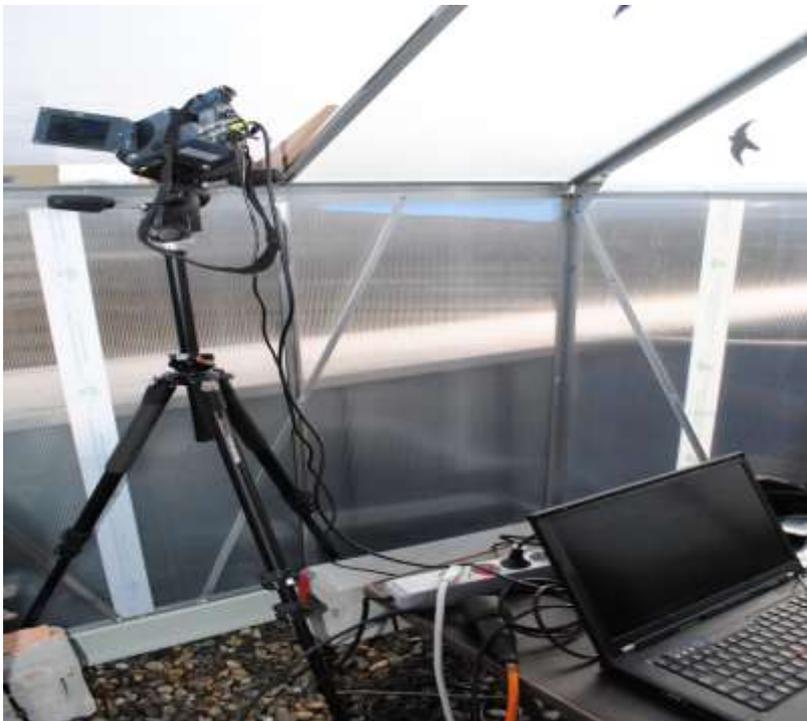
Fig. 4-4 – Infrared camera and laptop
